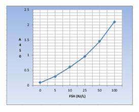
A typical std curve (Plot linear graph Draw the best curve through the points. Do not use this for calculating sample values).
